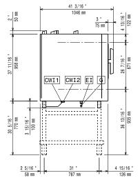
Cold Water inlet 1 (cleaning) CWII CWI2 Cold Water Inlet 2 (steam
